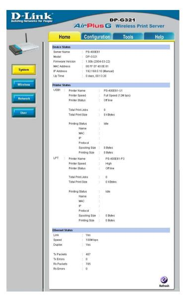
**Ethernet Status:** You can monitor the networking status in this field, including the network connection, speed, and the packets status.
